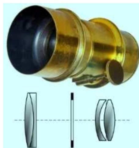
Figure 1. Petzval lens (objective). The first photographic portrait objective lens in the history of photography [18] . Image credit: Szöcs Tamás.
